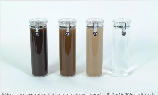
Water samples from a system that has been treated with EnwaMatic®. Day 1 to 30 from left to right.
